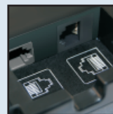
USB and TCP/IP USB plug and play. Easy data transfer. TCP/IP connection for multiple units in one network.
