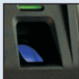
Optical fingerprint sensor New generation fully sealed, waterproof and dustproof fingerprint sensor. Unique finger positioning design.
